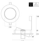
**Specifications Any Lamp Recessed Spot Circular Tiltable White | Cutout 75mm - GU5.3 Socket**
